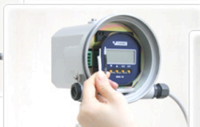
Pass the cable through the entry.
