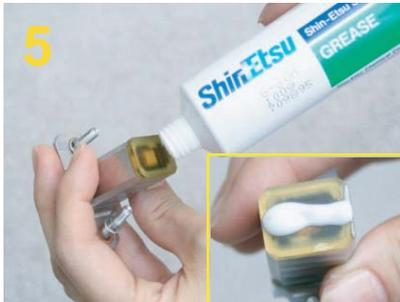
Put couplant onto surface of transducer as photo
