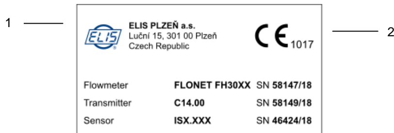
Example of the main meter plate
