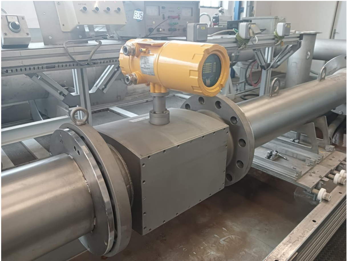
Fig. No. 8 Flow meter during tests on the test stand
